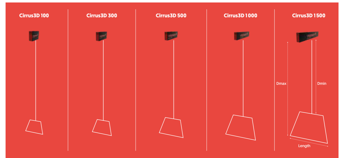
Dmin and Dmax are the minimum and maximum distance between Cirrus3D and scanned volume
