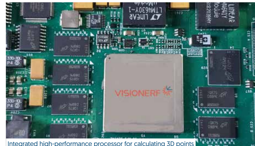
Integrated high-performance processor for calculating 3D points
